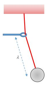
A crude demonstration is a simple pendulum with a string of variable length, for example (see figure) one hanging from a fixed support, but the string passing through a small loop that can be moved vertically to change the effective length.
