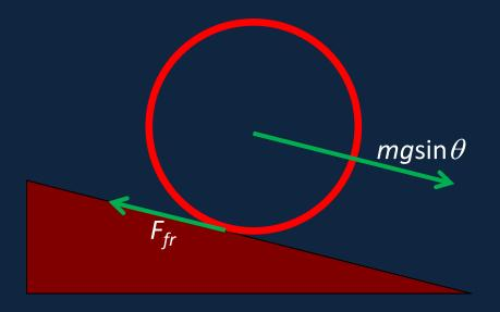
The only force having torque about the center of the hoop (its CM) is the frictional force: the total gravitational force and the normal force both act through the center.
