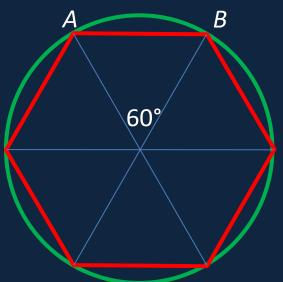
The straight line distance from A to B is one side of an equilateral triangle, exactly one radius, the arc from A to B is a bit further—so 60° is a little more than one radian.
