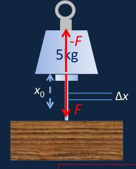
Weight hits nail with speed  $v_0$
