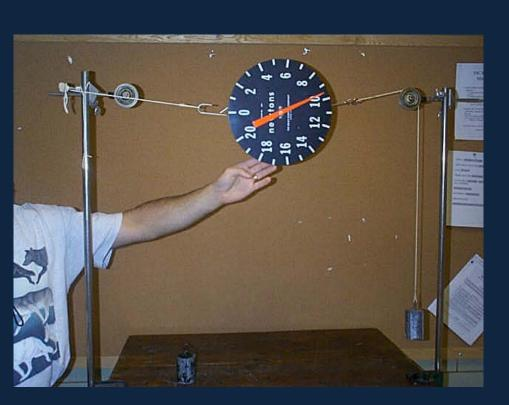
Suppose the looped end of the string is taken from the hook, put over the pulley, and a one kg mass is hung from that end too.
