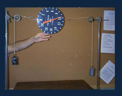
• The tension in the string is the weight of one kg, 9.8N. In the first case, the string was pulling the hook with 9.8N force, and the hook was pulling right back!
