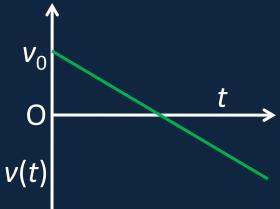
• The slope of the line is the acceleration a = -g.
