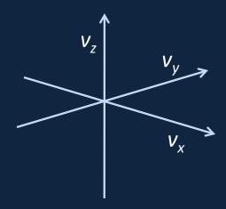
One dot in this 3D space would represent the velocity of one molecule at an instant.
