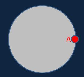
Initially, the man has moment of inertia  $mR^2$ , the turntable  $2mR^2$ . Finally, the man has negligible moment of inertia, so the total I decreases by a factor of 2/3, to conserve angular momentum (ther are no external torques)  $\omega$  increases by 3/2.
