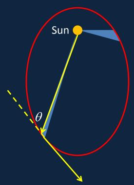
The base of the thin blue triangle is a distance v along the tangent. The height is the perp distance of this tangent from the Sun.
