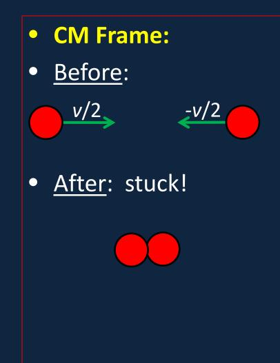
For the one-dimensional inelastic collision of a mass *m* moving at velocity *v* hitting and sticking to an initially stationary mass *m*, is the kinetic energy loss:
