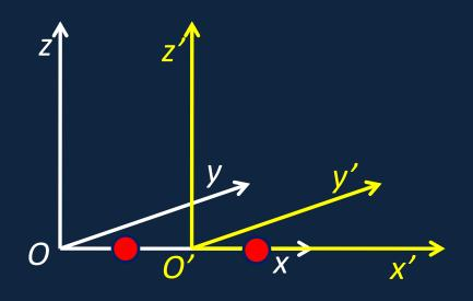
The fixed lab frame is in white. The CM frame is in yellow. The origin O' is always at the center of mass of the two balls. With no external forces, O' moves at constant velocity relative to O, so both frames are inertial, both conserve momentum.
