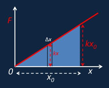
Area under this "curve" =½ base x height=  $\frac{1}{2}kx_0^2$  In fact, the total work done is the area under the force/distance curve for *any* curve: it's a sum of little areas  $F\Delta x$  corresponding to work for  $\Delta x$ .
