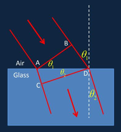
The wave front AB is perpendicular to the ray's incoming direction, CD to the outgoing—hence angle equalities.
