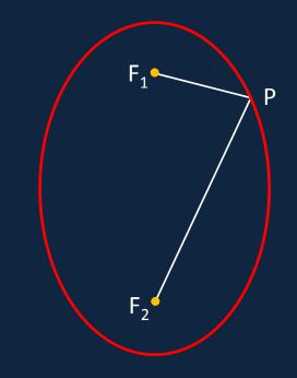
You can draw an ellipse by fixing the ends of a piece of string at A, B then, keeping the string tight, loop it around a pencil point at P and move the pencil around on paper.
