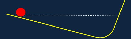
one steep and one shallow, and a ball rolling to the bottom would have the same speed from either side.
