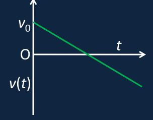
• The slope of the line is the acceleration a = -g.
