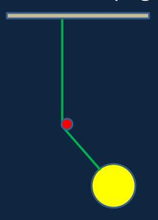
The pendulum will now move around a tighter arc on the right-hand side.
