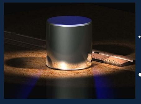
The unit of mass is the kilogram, defined as the mass of a chunk of platinum in Paris, shown here.
