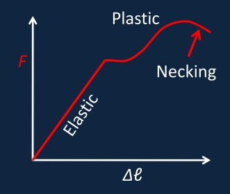
The shape of the curve in the plastic region differs from one substance to another—just before breaking, narrowing often occurs at one place : "necking".
