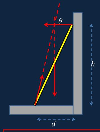
Warning: this trick saves working with components, but <u>does NOT</u> work if there are more than three forces! (Someone on the ladder.)
